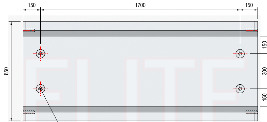
4 x 2.5t Lifting Pin x 55mm long (factor of safety x 3).
