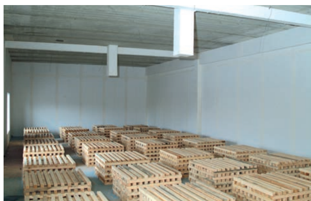
BRE's full-scale tests in 2006 demonstrated extremely good performance of the 200mm deep hollowcore floor plate.
